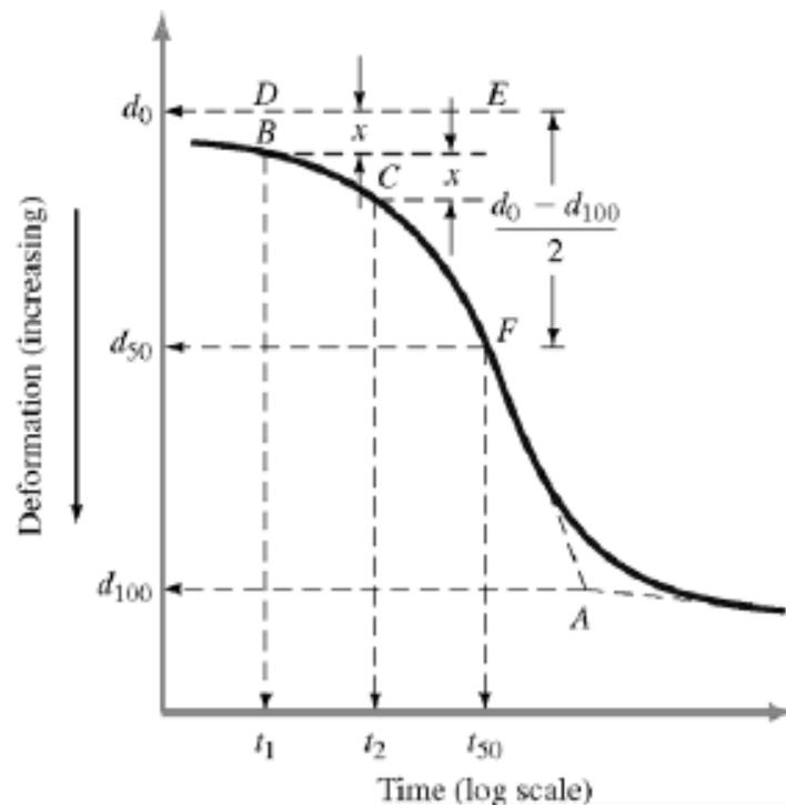
1. Extend the straight line portion of primary and secondary consolidations to intersect at Point A. Point A represents  $d_{100}$  (Deformation at 100% primary consolidation).
