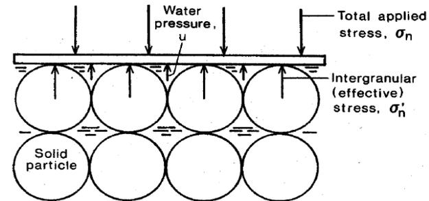
Fig. 2.10. Intergranular (effective) and water pressures in a saturated soil.
